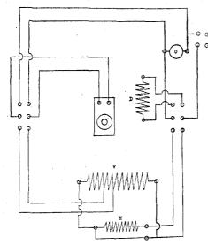
Fig. 2.—Potentiometer circuits.
