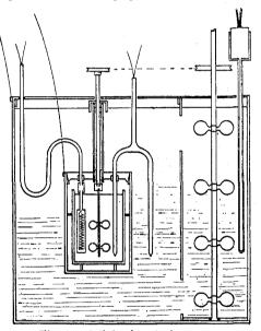
Fig. 1.---Adiabatic calorimeter.
